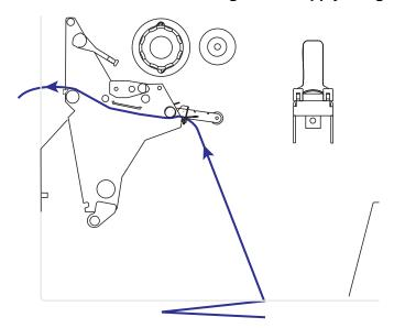
Figure 17 • Bottom Feed Without Using Media Supply Hanger
